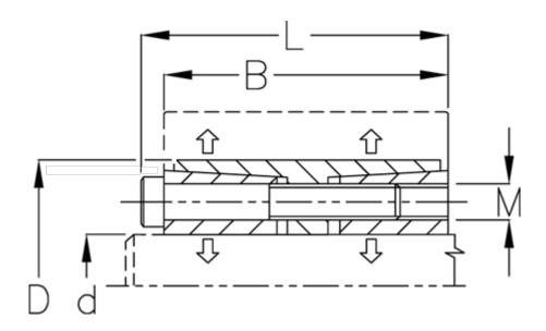
B mm = 202= 400 d H8 mm D mm = 495Fit tolerance = Aksel h8, Nav H8
